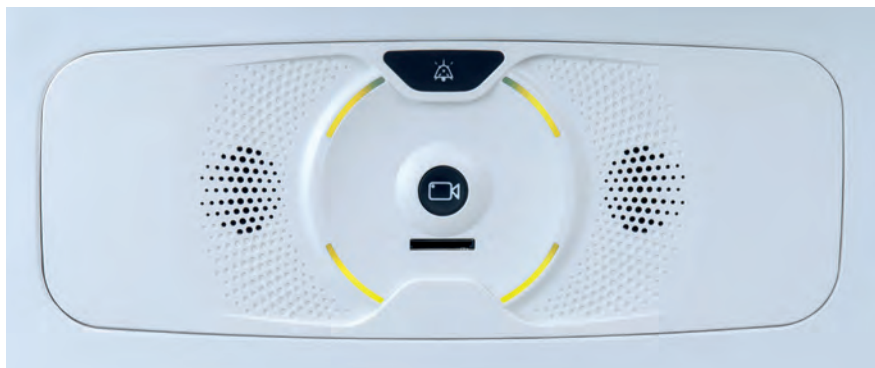
Figure 20.3 Status halo on the surgeon console indicating a console alarm
