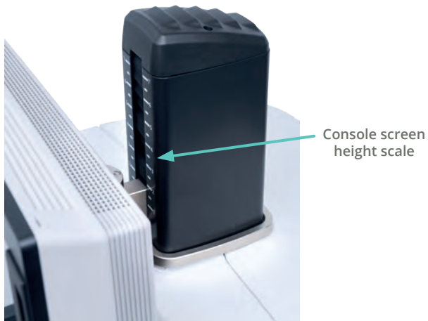
Figure 13.5 Height scale on surgeon console screen
