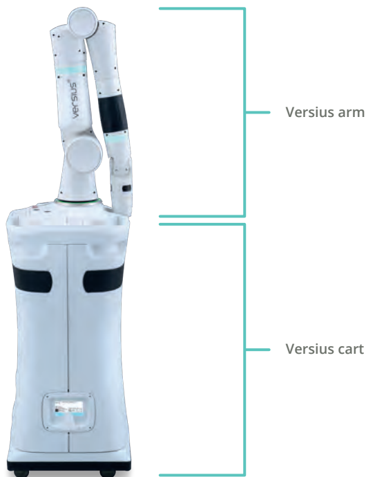
Figure 2.11 The arm and cart labelled on the Versius Bedside Unit
