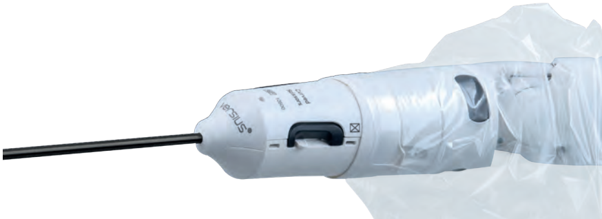
Figure 15.2 Red marks on drape cap are obscured when instrument is securely attached
