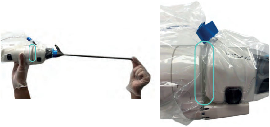
Figure 14.2 Support the arm near the camera head and grip the end of the endoscope; gap between the camera head and the arm is open
