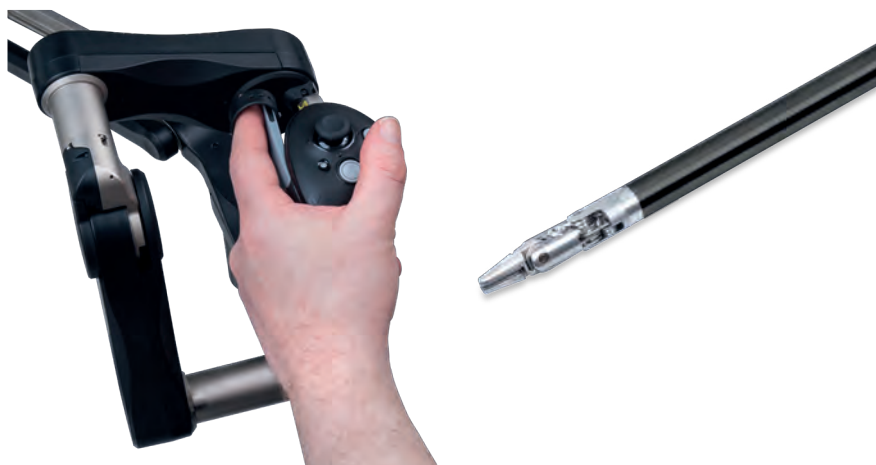
Figure 18.3 Hand controller with jaw control in neutral position
