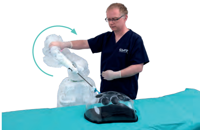
Figure 17.3 Instrument inside the port with an arrow to indicate circular arc trajectory
